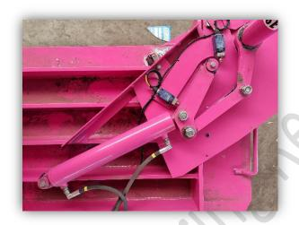
Hydraulic door lock & unlock system operated by a push of a button. Safety limit switches fitted so the machine can detect if the door is locked or unlocked.
