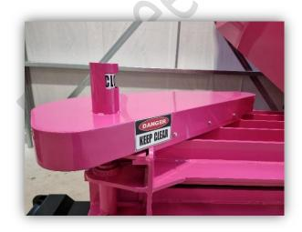
Covered by a removeable guard for ease of greasing. Fitted with an open / close window.
